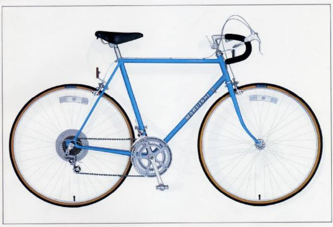
FRAME: FRAME SIZES: 19°, 21°, 23°, 25° 8-27° Monsi19° & 22° Ladles, MAIN TUBING: Chromemoly plain-gauge tube. LUGS: Nikko cover cut. SEAT & CHAIN STAYS: Hi tension steel. FRONT FORK: Hitension steel. FORK CROWN: A-OW, ENDS: Stamped. BRAZE-ONS: Brake cable tunnels on top tube, 3 rings for Ladles/Derailleur cable stop on chainstay/ Shift lever stop on down tube. HEADSET: Nikyo 65-4, TIRES: IRC 27° × 1-1/4° gumwall 90 psi, Schrader valves.
